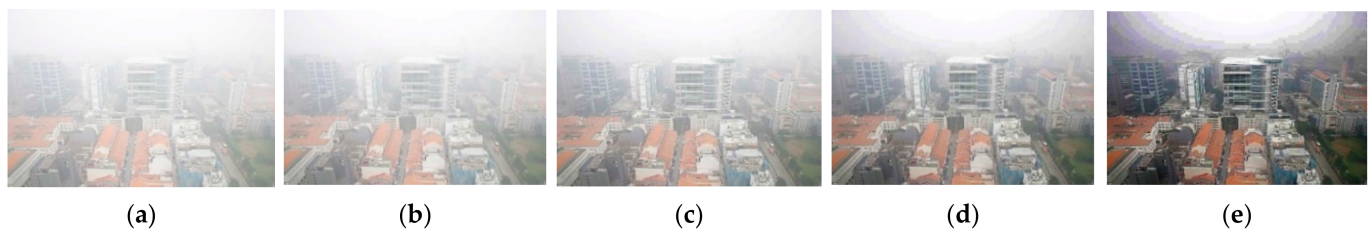
Figure 7. The effects of haze control parameter \omega : (a) input hazy image, (b) recovered image ( \omega = 0.25 ), (c) recovered image ( \omega = 0.5 ), (d) recovered image ( \omega = 0.75 ), and (e) recovered image ( \omega = 1.0 ).
