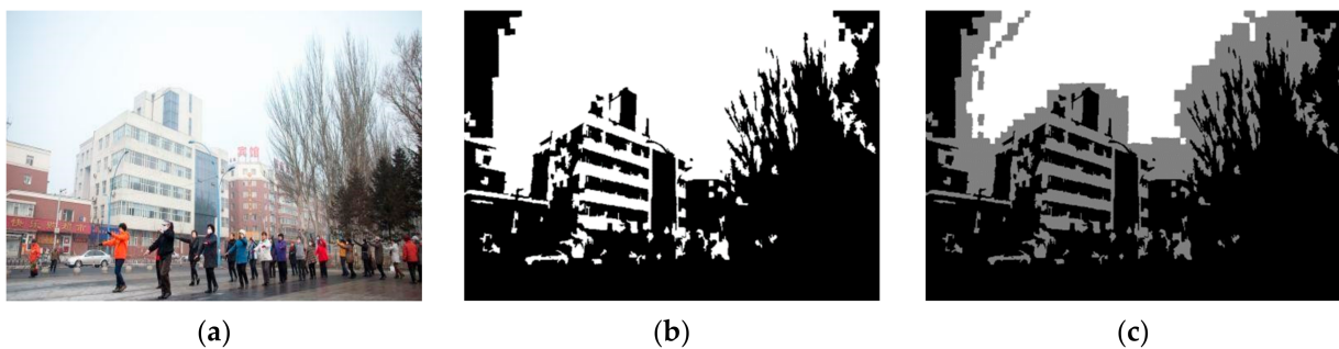
Figure 4. Region separation based on the atmospheric light A : (a) input image, (b) the result of Equation (11), and (c) proposed method.
