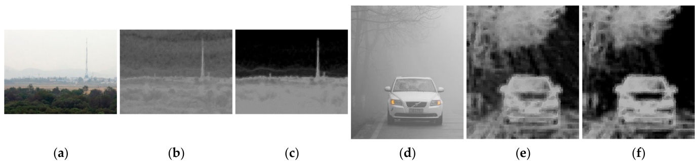
Figure 8. Comparison of local image entropy: (a,d) input image, (b,e) entropy calculated from input image, and (c,f) entropy calculated from gradient of image.
