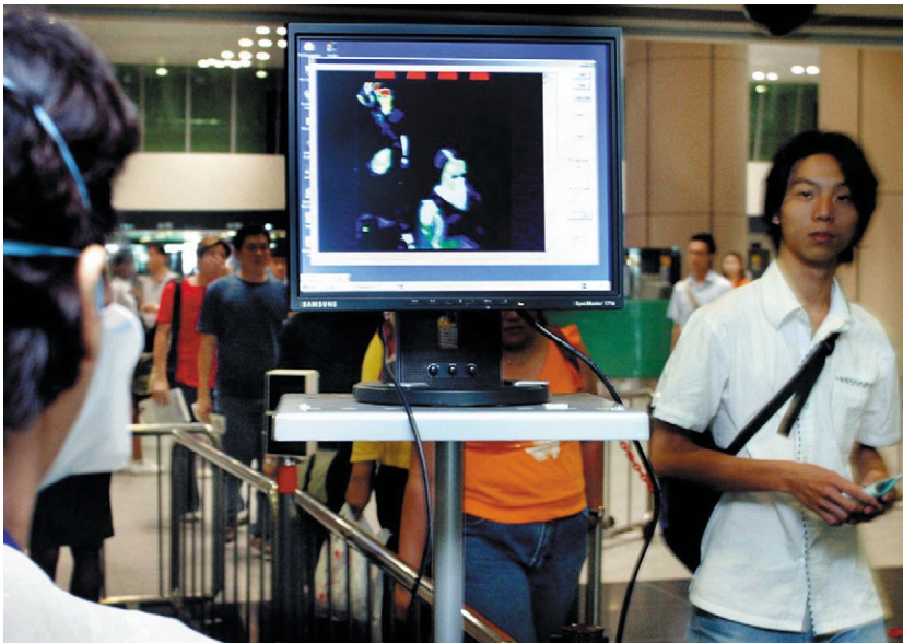
Figure 2. A typical infrared body-temperature screening device used in airports and at the entrance of office buildings in Taipei. Passengers walk through at a usual pace. The faces of passengers whose body temperatures are higher than 38°C show up as a red image on the screen.
