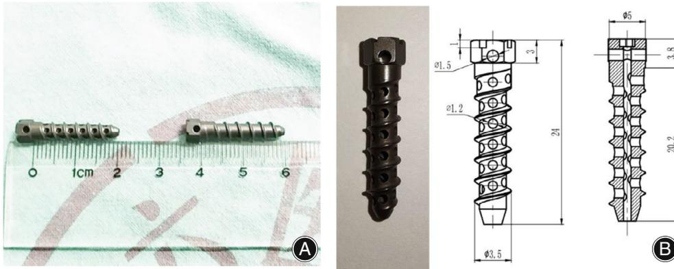
**Fig. 1** The structure of the novel lateral hole pedicle screw (LHPS) and the solid pedicle screw (SPS). (A) The LHPS and the SPS. (B) The diagram of the LHPS (Dimension: mm)
