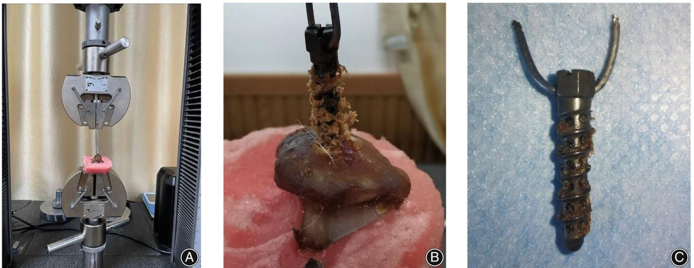
**Fig. 5** (A) The pull-out test for the lateral hole pedicle screw (LHPS). (B) LHPS was pulled out with part of the bone adhere. (C) Lateral holes and inner spaces were filled with cancellous bone
