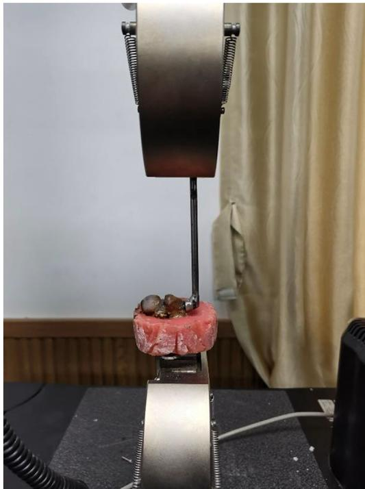
**Fig. 3** Cyclic bending test. Loading was applied to the head of the screw through the rod in a vertical direction to the screw axis
