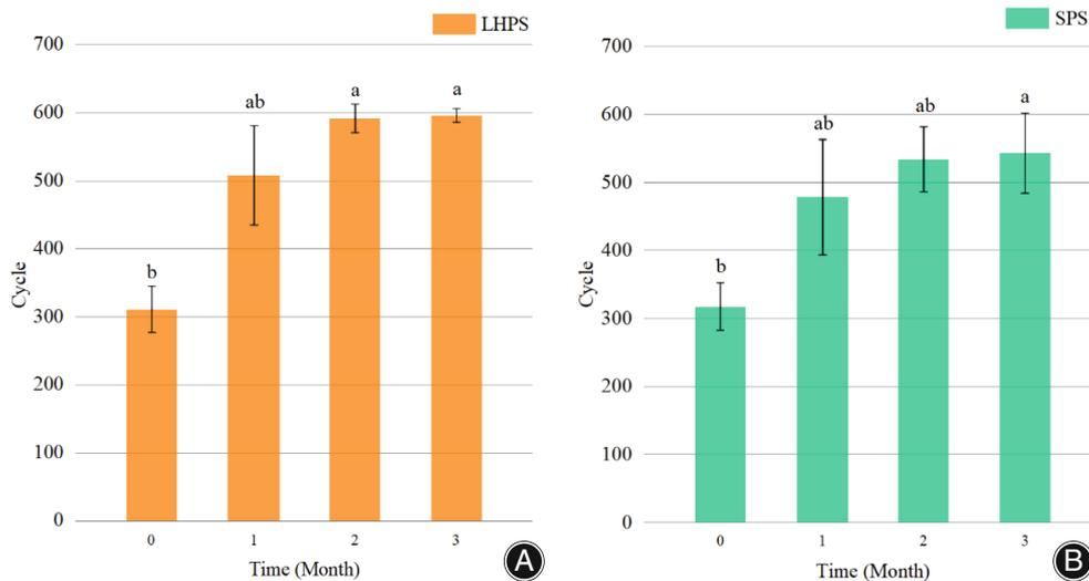
**Fig. 7** The average number of cycles for lateral hole pedicle screws (LHPSs) and solid pedicle screws (SPSs) at different time points in the cyclic bending tests. Error bars represented mean  $\pm$  SD. The difference between groups was analyzed using the Friedman and the *post hoc* multiple comparisons test. A significant difference is indicated by different letters,  $P < 0.05$
