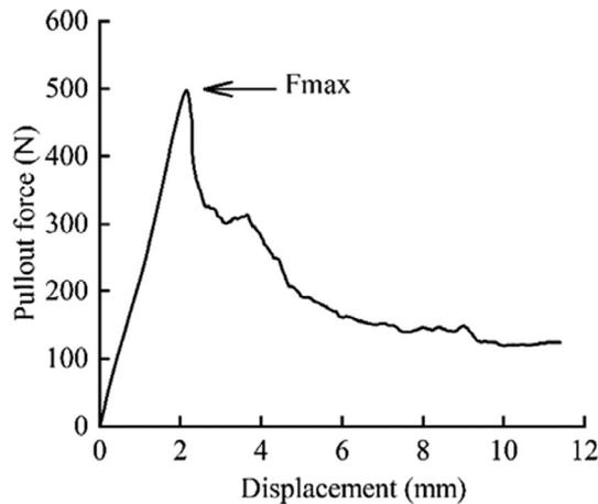
**Fig. 4** The force-displacement curve after the axial pull-out test of the lateral hole pedicle screw (LHPS). The maximum pullout strength ( $F_{max}$ ) was defined as the inflection point at which the load hits its peak and drops sharply as displacement increases
