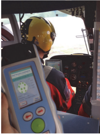
FIGURE 3: The Infrascanner 2000 was implemented in a Dutch helicopter emergency medical service (HEMS). For safety reasons, the device was tested prior to implementation for possible interference with existing on-board medical equipment, electronics, and avionics of the helicopter (Eurocopter EC-135, Airbus industries) both on ground and during flight.
