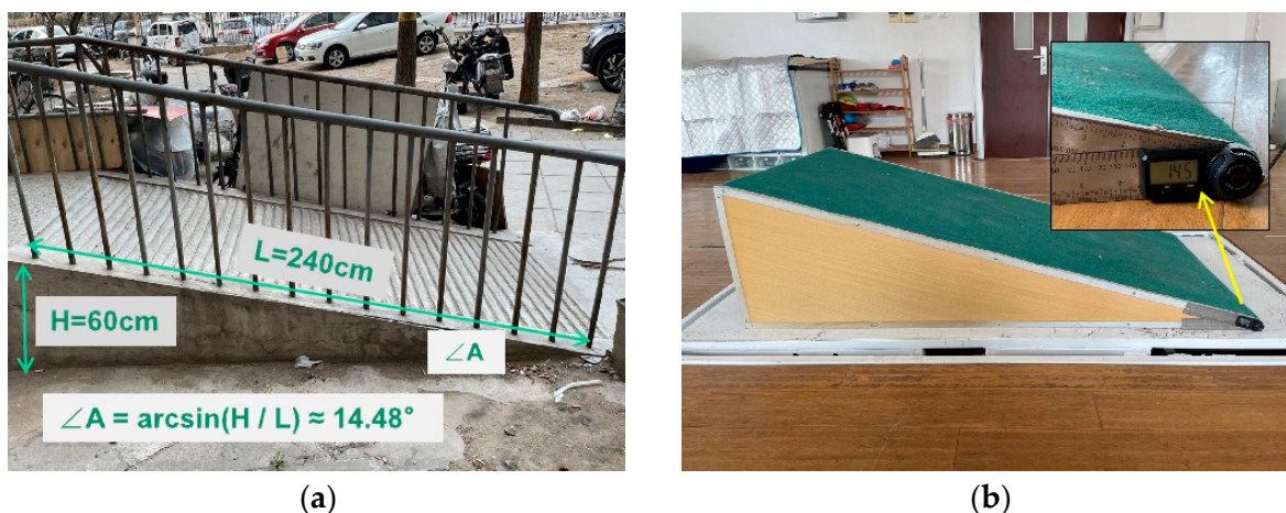
Figure 2. The degree of slope in the barrier-free environment: (a) measured in an old community, and (b) simulated in the experimental environment.
