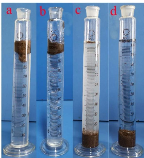
**Figure 11.** Result of proppant suspension measurements, (a) Fluid-1, (b) Fluid-2, (c) guar gum, and (d) linear glue.
