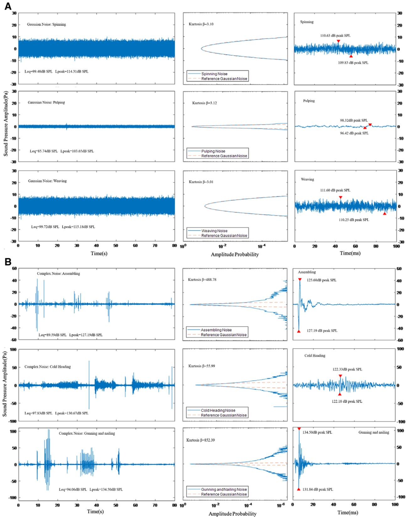
Fig. 1. Waveforms (left), amplitude probabilities (middle), and peak SPL distributions (right) from 13 typical industrial noises. (A) Spinning, pulping, and weaving; (B) assembling, cold heading, and nail gunning; (C) forging, metal processing, and woodworking; (D) polishing, punching, stamping; and (E) welding.
