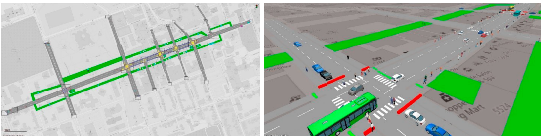
Fig. 1. Isometric view of the Spring Garden Road Fig. 2. Microsimulation of vehicles and pedestrians
