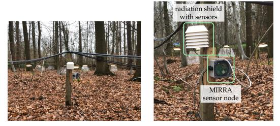
**Figure 2.** Sensor node in the experimental set-up, consisting of a sensor board (square block), radiation shield (white) and ground probe. This set-up is located in the "Aelmoeseneie" forest in Gontrode, Belgium (50.98° N, 3.80° E).
