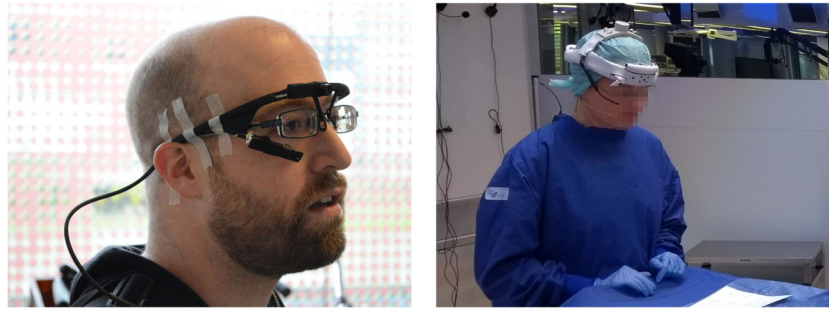
Fig. 1 Head-worn eye trackers. Two examples of extreme measures taken by researchers to prevent slippage of a head-worn eye tracker: tape ( left panel , courtesy of Jeroen Benjamins) and a helmet mount ( right panel , courtesy of Shahram Eivazi)
