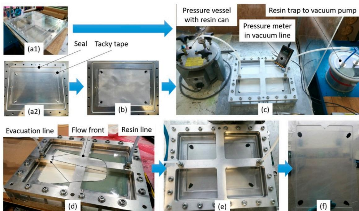
**Figure 5.** The RTM setup and its processing states: (a1) upper PMMA-mold, (a2) lower aluminum mold, (b) reinforcement in the cavity, (c) assembled mold, (d) resin injection, after 24 h of (e) cure, and (f) the demolded part.
