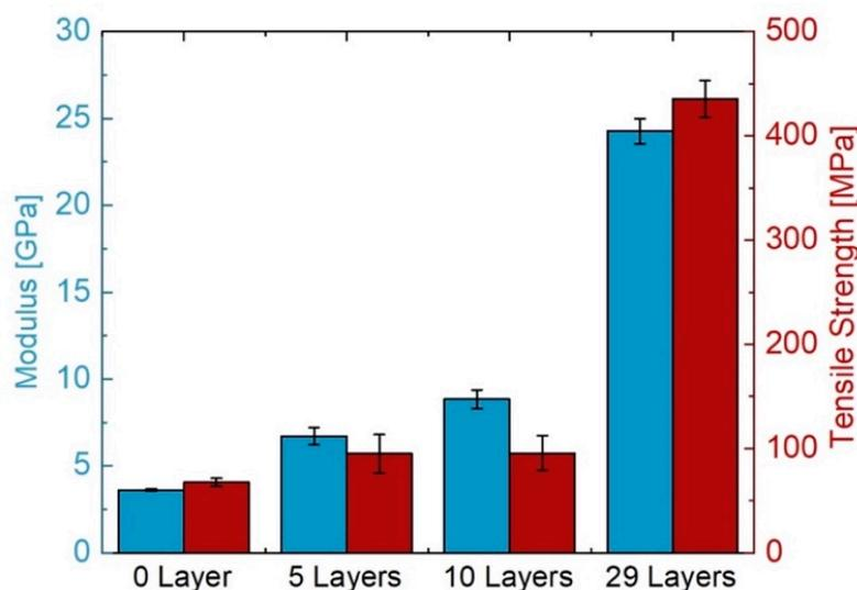
**Figure 10.** Mechanical properties of transparent composites in comparison to the unfilled resin (0 Layer).
