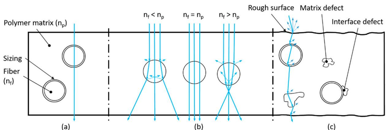
**Figure 1.** Optical effects of an incident ray permeating a tGFRP with (a) ideal properties: matching RI, smooth surface and no defects, (b) different levels of RI mismatch between polymer ( $n_p$ ) and fiber ( $n_f$ ) [14], and (c) realistic properties including defects that decrease the optical quality.
