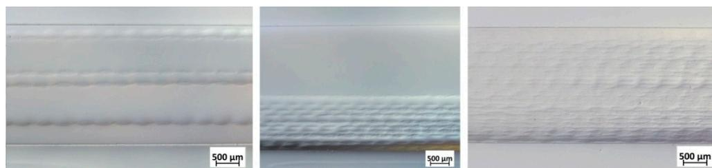
**Figure 6.** Light microscope images showing the cross-section of the composite samples manufactured via RTM with 5 (left), 10 (middle), and 29 layers (right) of E-glass fabric in a thermoset polymer matrix.
