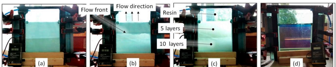
**Figure 4.** The L-RTM vacuum infusion states on the example of a preform (a) pre-infusion (b) during infusion (c) after infusion and set for cure (d) after 24 h of curing, with resin only (up), 5 layers (middle) and 10 layers (below).
