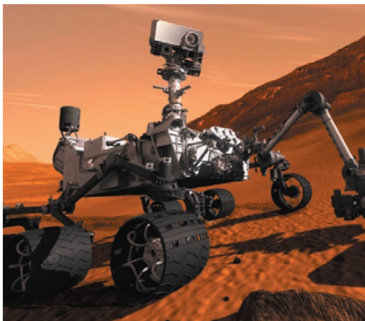
FIGURE 3-5: An SCR could be a build-to-print copy of the MSL Curiosity rover with a new science payload and a sample collection and caching system (Source NASA).
