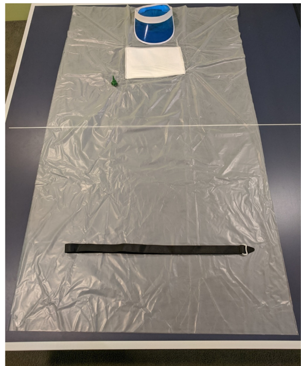
Figure 1. Final design disposable isolation device: integrated oxygen nozzle (green), integrated N-95 filter patch (white), internal visor (blue), and Velcro belt (black) on background torso bag with one open end. (Color version of figure is available online.)
