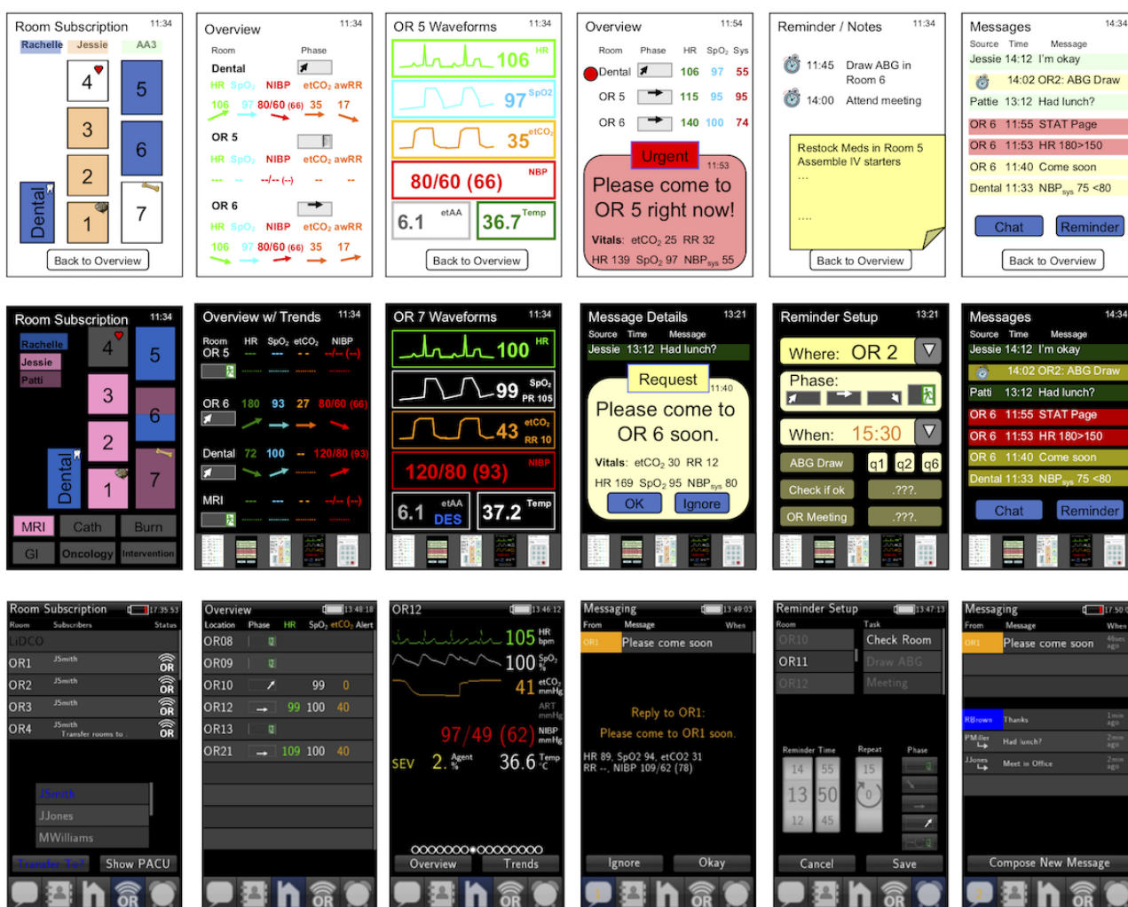
Figure 1. Progression of the telePORT app from initial concepts (top row), to intermediate prototype re-designed after user feedback (middle row), to final app (bottom row). The app features shown are: room subscription screen (first), overview screen (second), waveform/numeric detail screen (third), help request screen (fourth), reminder setup (fifth), and messaging overview screen (sixth).
