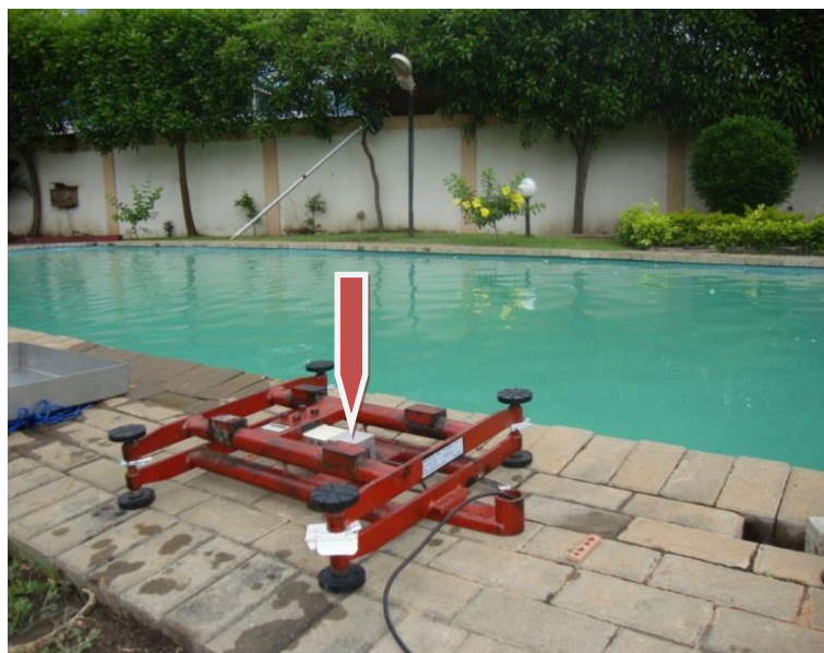
Figure 1 Load cell within metal framework of the weighing scale (Red Arrow).
