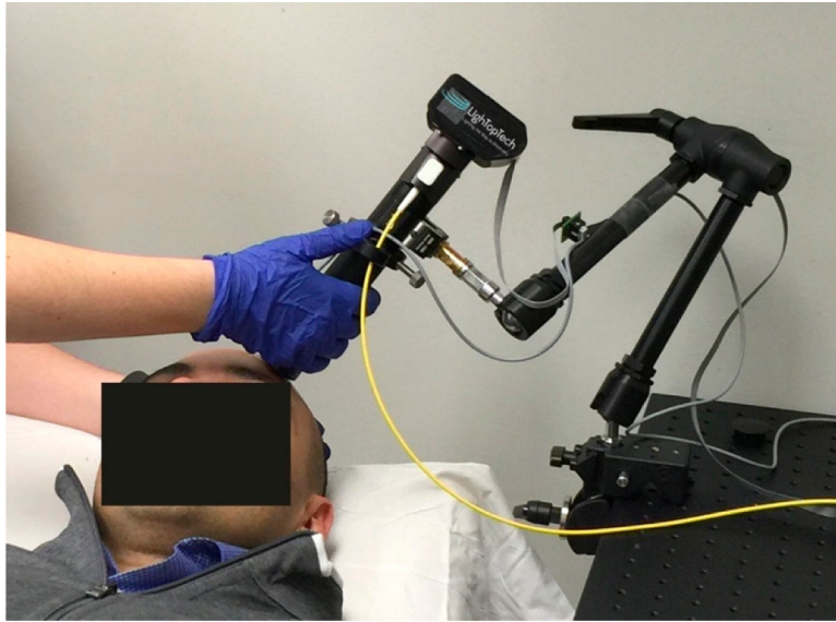
Figure 6. Handheld GDOCM microscope. A mechanical arm can be used to reduce operator hand tremor.
