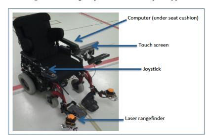
**Figure 1.** Intelligent power wheelchair prototype.
