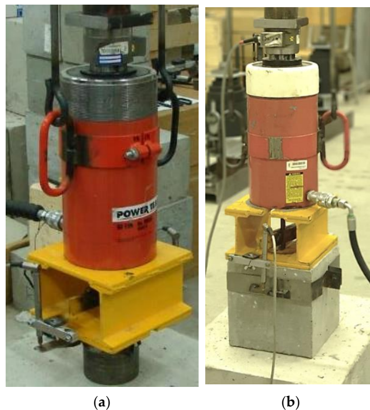
Figure 7. (a) Test with a steel base specimen; (b) Test with a concrete base specimen.
