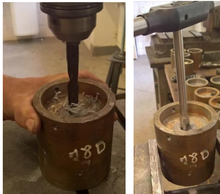
Figure 8. Steel base specimen restoration cleaning procedure.
