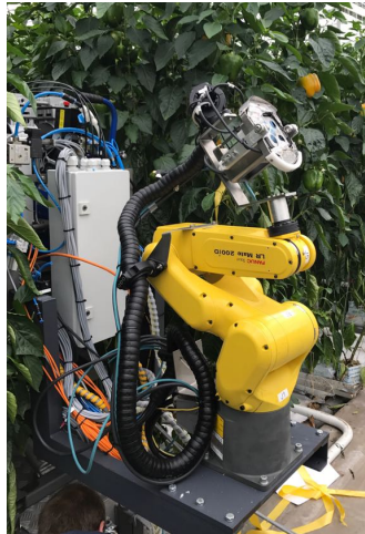
Figure 5. Experimental setup including a robotic arm, equipped with an RGBD camera and an illumination rig.
