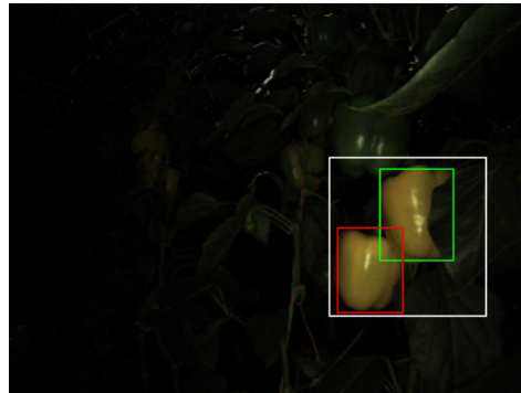
Figure 8. Example of a clustered detection: the detected area ( white ) overlaps both a pepper considered to be a true positive detection ( green ) as well as one considered a false negative detection ( red ).
