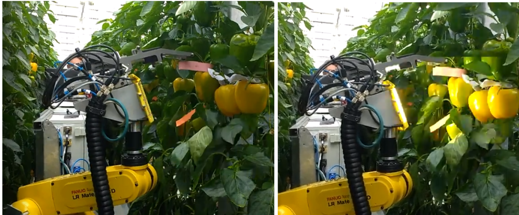
Figure 1. Experimental setting for FNF image acquisition; the same image is taken twice, with (right) and without (left) artificial light.
