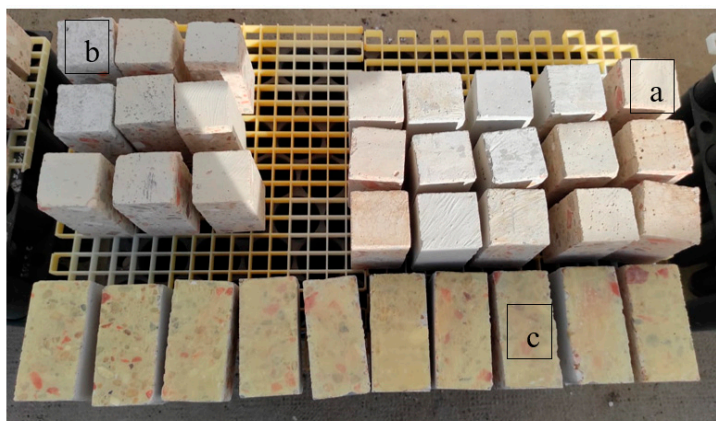
Figure 1. The water drop absorption test specimens: (a) outdoor specimens from the test performed to compare indoor and outdoor treatments; (b) specimens used to analyze the effect of the reapplication of treatments; (c) specimens used to evaluate treatment effects on vertical exposure.
