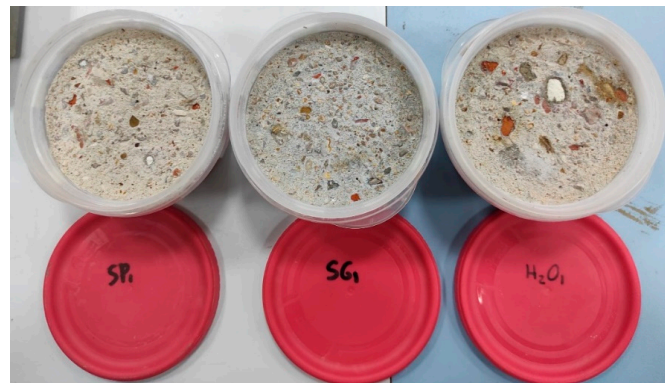
Figure 6. Surfaces of control, SP and SG specimens after the freeze–thaw test.
