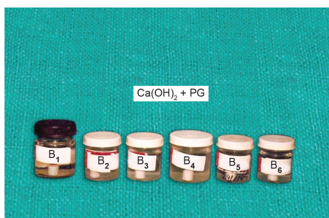
Fig. 3: Six bottles containing 40 ml of distilled water with porcelain caps immersed into it having a paste of a \text{Ca}(\text{OH})_2 + \text{PG}
