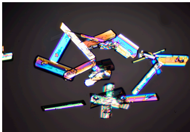
Figure 4. Polarized light microscopic picture at 40× magnification of Fondaparinux crystals formed from a water/ethanol solution.
