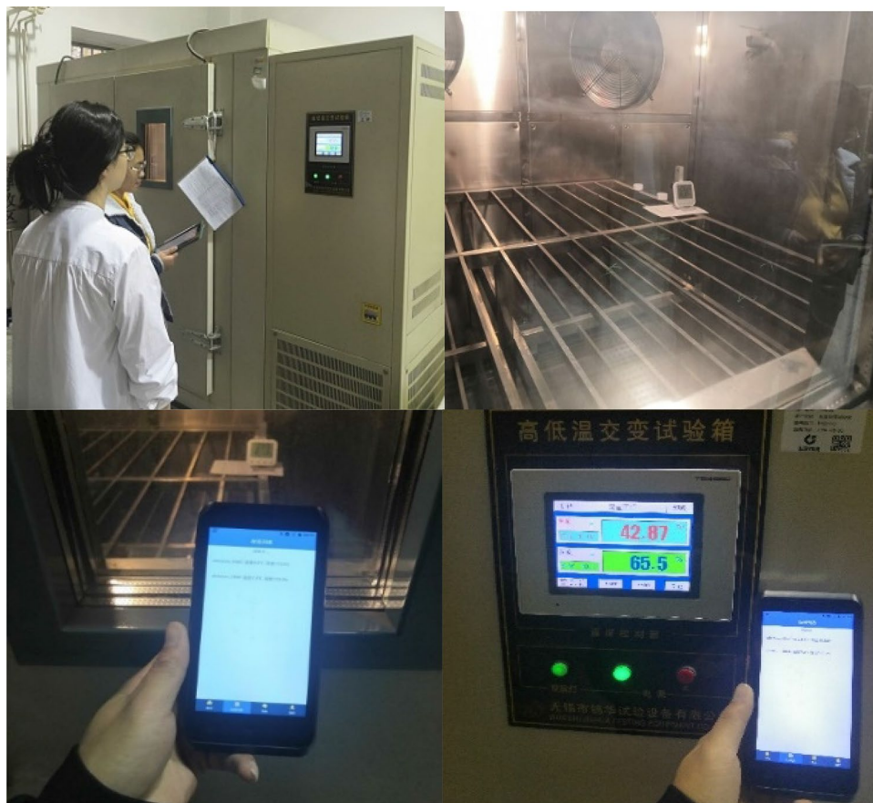
Figure 18. Test of temperature and humidity monitoring.
