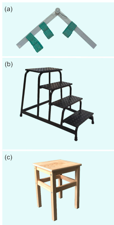
Figure 3. (a) Additional goniometer used during the calibration process, with Velcro straps and transparent lever arms that enabled positioning along anatomical lines, (b) portable aluminum staircase used for stair ascend and stair descend, (c) armless wooden stool used for sitting down and getting up.
