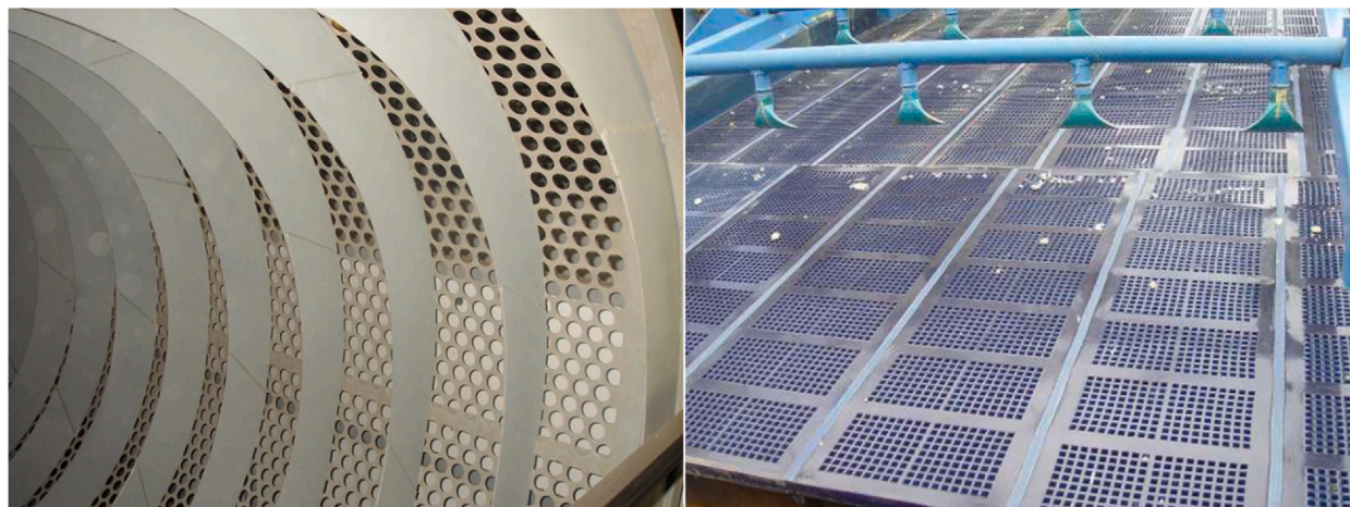
Fig. 1. Typical screens used in processing plants. On the left, a rotary drum screen, on the right, flat aluminum screen.
