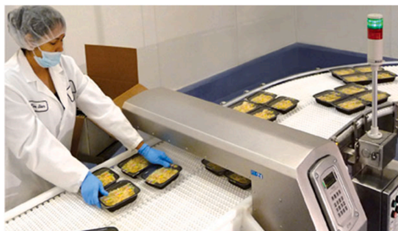
Fig. 3. Typical metal detector in food processing.
