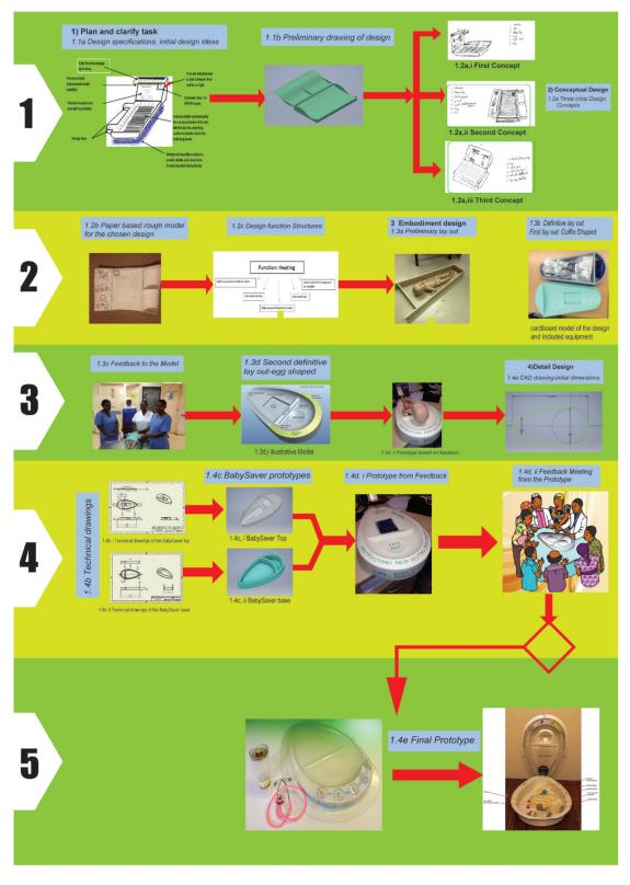
conceptual design, (3) embodiment design, and (4) detailed design. Figure 1 shows a summary of the design process specific to the BabySaver based on this framework [22].
