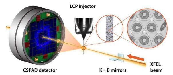
**Figure 1.** Experimental setup for serial femtosecond crystallography (SFX) data collection using an LCP injector. Microcrystals dispersed in LCP are injected as a continuous column of 20– $50~\mu m$  diameter and intersected with  $1.5~\mu m$  diameter pulsed XFEL beam focused by Kirkpatrick–Baez (KB) mirrors. Single pulse diffraction patterns are collected at 120~Hz using a CSPAD detector. (Adapted from Liu et al. [28]).
