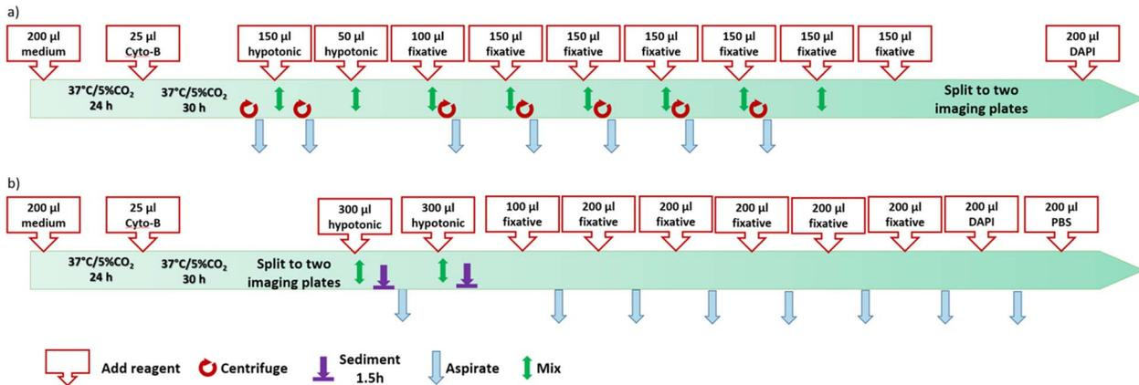
**Fig. 1.** Overall workflow of the a) accelerated and b) centrifuge-free accelerated CBMN assays developed for the RABiT II system. **Dispense:** adding the required amount of reagent. **Mix:** aspirate and dispense 200  $\mu\text{L}$  five times. **Centrifuge:** 1200 rpm/2 min. **Aspire:** aspire all liquid from about 1 mm above plate bottom—200  $\mu\text{L}$ , **Sediment:** leave plate on bench for 1.5 h.
