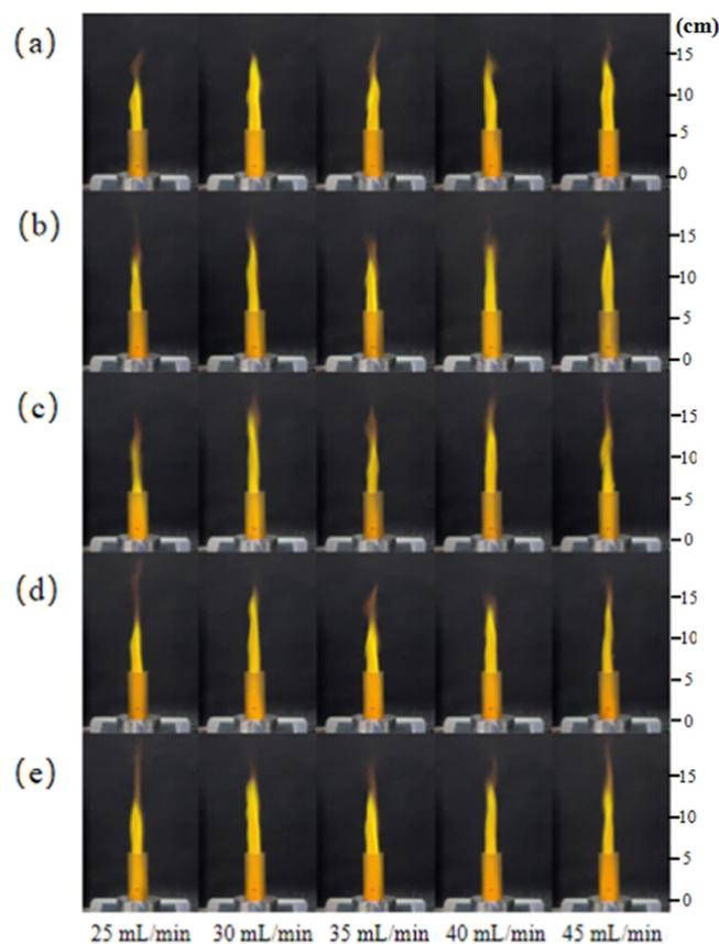
**Figure 6.** Jet flame images under different propellant flow rates at (a)  $t = 5$  s, (b)  $t = 10$  s, (c)  $t = 15$  s, (d)  $t = 20$  s, and (e)  $t = 25$  s after ignition.
