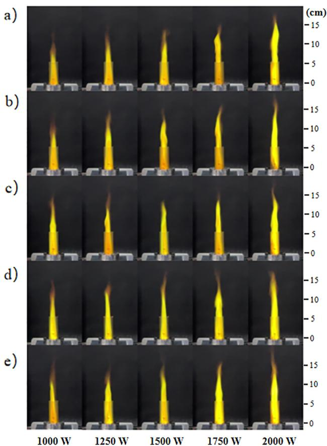
**Figure 2.** Jet flame images under different microwave powers at (a)  $t = 5$  s, (b)  $t = 10$  s, (c)  $t = 15$  s, (d)  $t = 20$  s, and (e)  $t = 25$  s after ignition.
