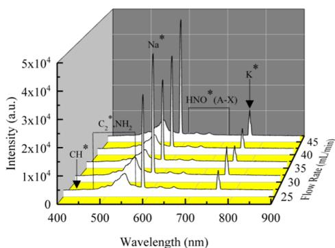
**Figure 8.** Corrected emission spectral distribution of the ADN-based liquid propellant jet flame obtained under different propellant flow rates.
