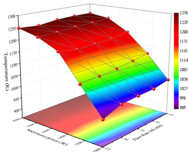
**Figure 10.** Temperature diagram of the ADN-based liquid propellant jet flame as a function of microwave power and flow rate in an atmospheric environment.
