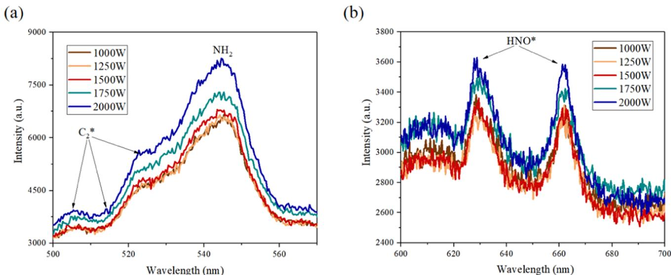
**Figure 9.** (a)  $C_2^*$  and  $NH_2$  emission bands of the ADN-based liquid propellant jet flame under different propellant flow rates. (b)  $HNO^*$  emission bands of the ADN-based liquid propellant jet flame under different propellant flow rates.
