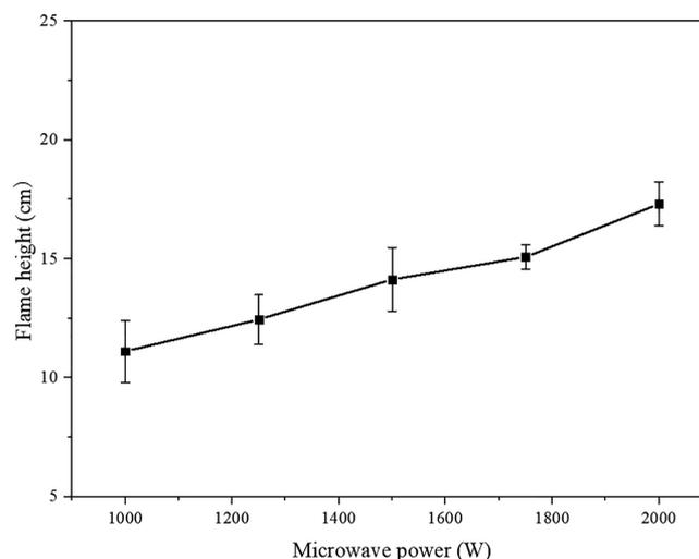
**Figure 3.** Average flame height of the ADN-based liquid propellant under different microwave power levels in an atmospheric environment; the error bars represent the approximate value.
