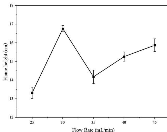
**Figure 7.** Average flame height of the ADN-based liquid propellant under different propellant flow rates in an atmospheric environment; the error bars represent the approximate value.
