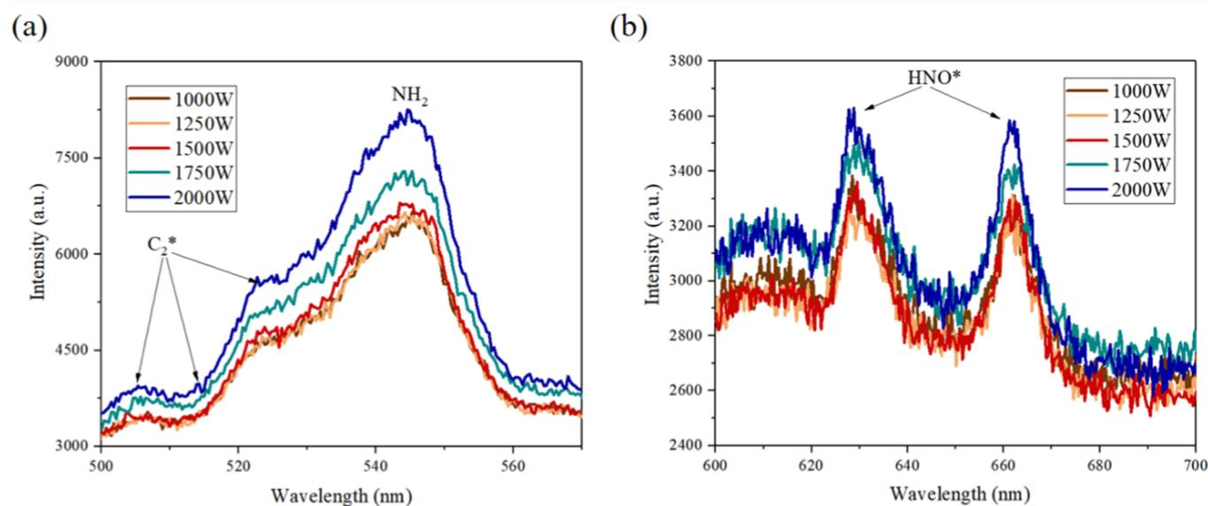
**Figure 5.** (a) C<sub>2</sub>\*, NH<sub>2</sub> emission bands of the ADN-based liquid propellant jet flame under different microwave power levels. (b) HNO\* emission bands of the ADN-based liquid propellant jet flame under different microwave power levels.
