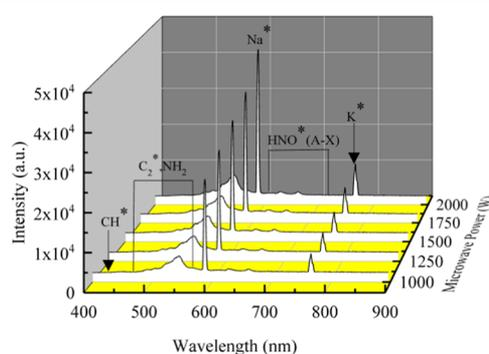
**Figure 4.** Corrected emission spectral distribution of the ADN-based liquid propellant jet flame under different microwave power levels.
