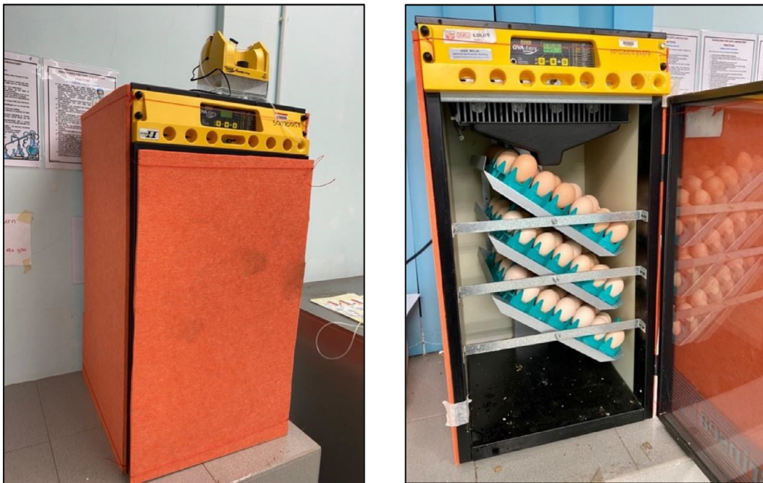
Figure 1. The external view: experimental incubators with acoustic padding isolation; internal view: incubator platform with automatic turning and the speaker placed in the incubator chamber.
