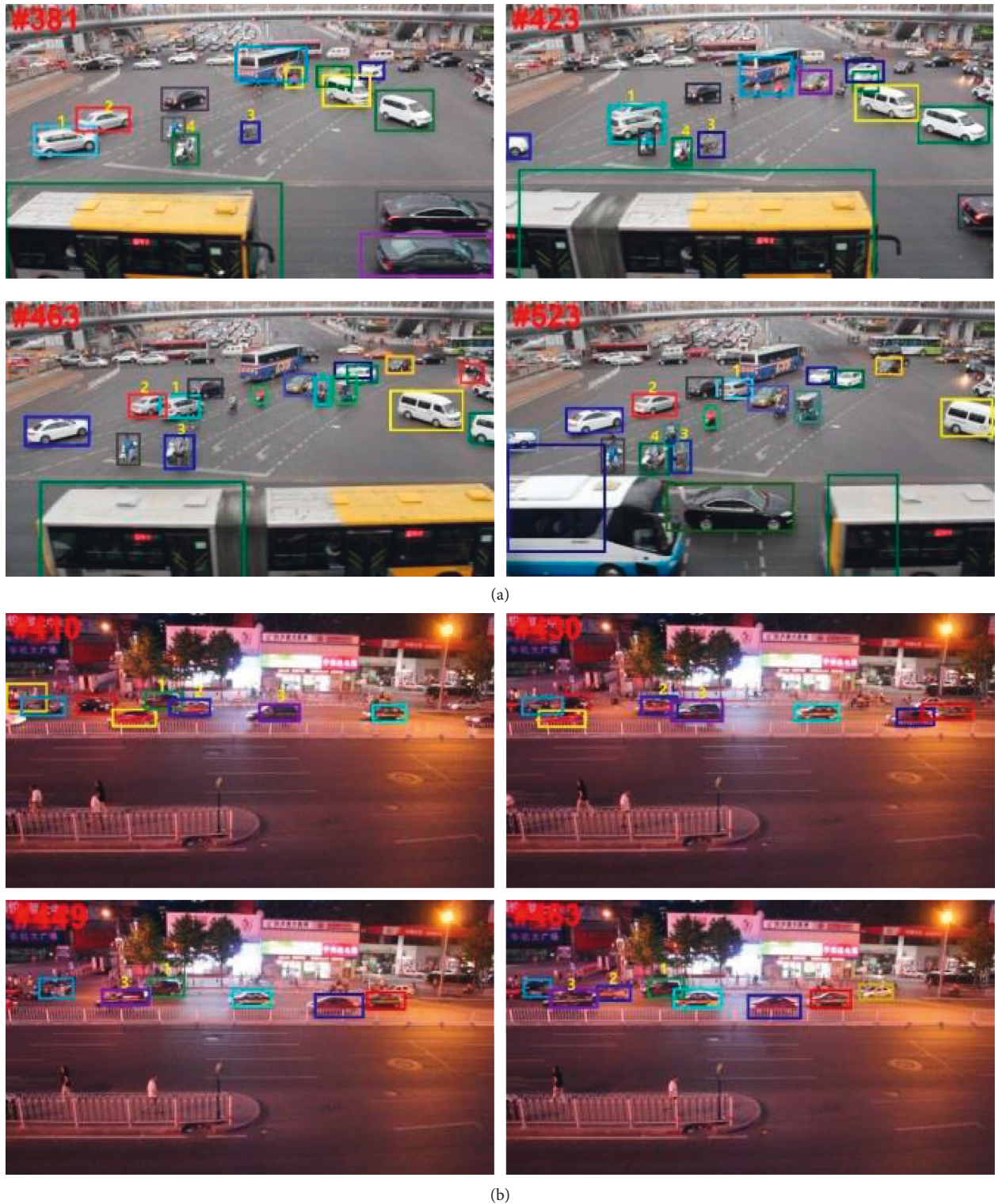
FIGURE 5: Tracking examples of the proposed method from UA-DETRAC dataset. (a) Sequence MVI_40853. (b) Sequence MVI_40763.
