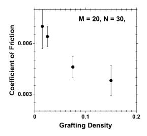
**Figure 8.** Coefficient of friction versus grafting density ( $\rho$ ) for M = 20, N = 30 in the presence of a good solvent. Here, the coefficient of friction is calculated from the slope of shear stress against normal stress in Figure 7 (so-called Approach A) and not for a particular velocity (so-called Approach B).
