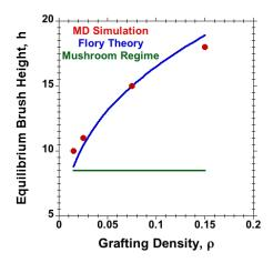
**Figure 2.** Equilibrium-brush height (*h*) versus grafting density ( $\rho$ ) for M = 20 flexible chains with N = 30 under good-solvent conditions. The  $\rho$ -independent reference result for the mushroom regime is marked by the horizontal line. Flory results according to Section 3.3.
