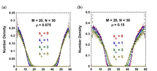
**Figure 3.** Polymer concentration profiles for non-interacting, opposing brushes at two grafting densities (a)  $\rho = 0.075$  and (b)  $\rho = 0.15$  for chains of various values of bending stiffness  $k_b$  (M = 30 chains with N = 30 on each side). Brush heights shown in Figure 4 are extracted from these profiles.
