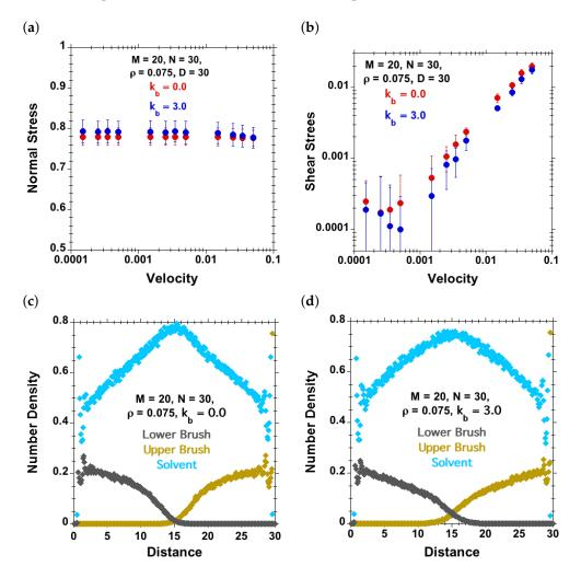
**Figure 11.** Effect of chain stiffness (red dots for  $k_b = 0$  and blue dots for  $k_b = 3$ ) for M = 20, N = 30,  $\rho = 0.075$ , D = 30 and good-solvent quality. (a) Normal stress against velocity; (b) shear stress against velocity; (c–d) concentration profiles of solvent (cyan), lower polymer-chains (grey) and upper polymer-chains (brown) for (c)  $k_b = 0$  (flexible) and (d)  $k_b = 3$  (semiflexible).
