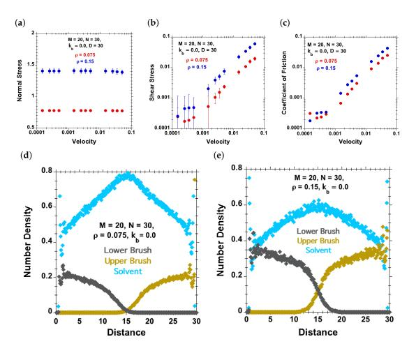
**Figure 9.** Effect of grafting density (red dots for  $\rho = 0.075$  and blue dots for  $\rho = 0.15$ ) for M = 20, N = 30,  $k_b = 0$ , D = 30 and good-solvent quality. (a) Normal stress against velocity; (b) shear stress against velocity; (c) coefficient of friction against velocity (Approach B); (**d**–**e**) density profiles of solvent (cyan dots), lower polymer-chains (grey dots) and upper polymer-chains (brown dots) for (**d**)  $\rho = 0.075$  and (**e**)  $\rho = 0.15$ .
