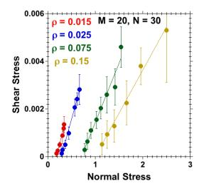
**Figure 7.** Effect of grafting density for M = 20, N = 30,  $k_b = 0$  and good-solvent quality; shear stress against normal stress for systems with grafting densities  $\rho = 0.015$ , 0.025, 0.075 and 0.15. The stresses were calculated over a range of separations, D, such that D < 2h for each data point. Straight lines represent linearly interpolated fits; their slopes are shown in Figure 8.
