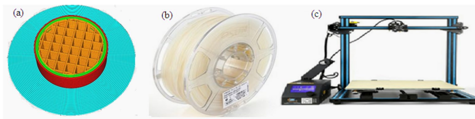
Figure 1. Machines used in 3D-printing, (a) horizontal cross section of the designed shape, (b) Esun Filaments and (c) 3D-printing machine model Creality CR10.
