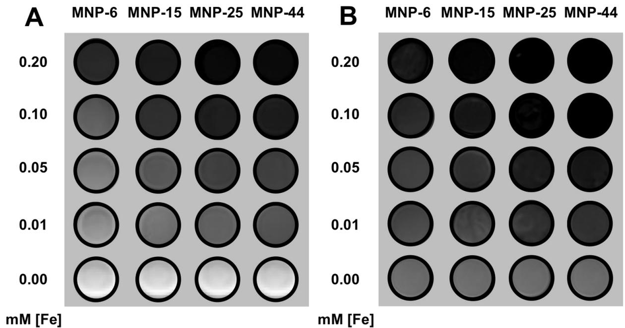
**Figure S3:** Series of  $T_2$ -weighted images of NPs solutions in water (A) and 2% agarose (B) acquired at  $TE = 48$  ms and concentrations ranging from 0.00 to 0.20 mM Fe.
