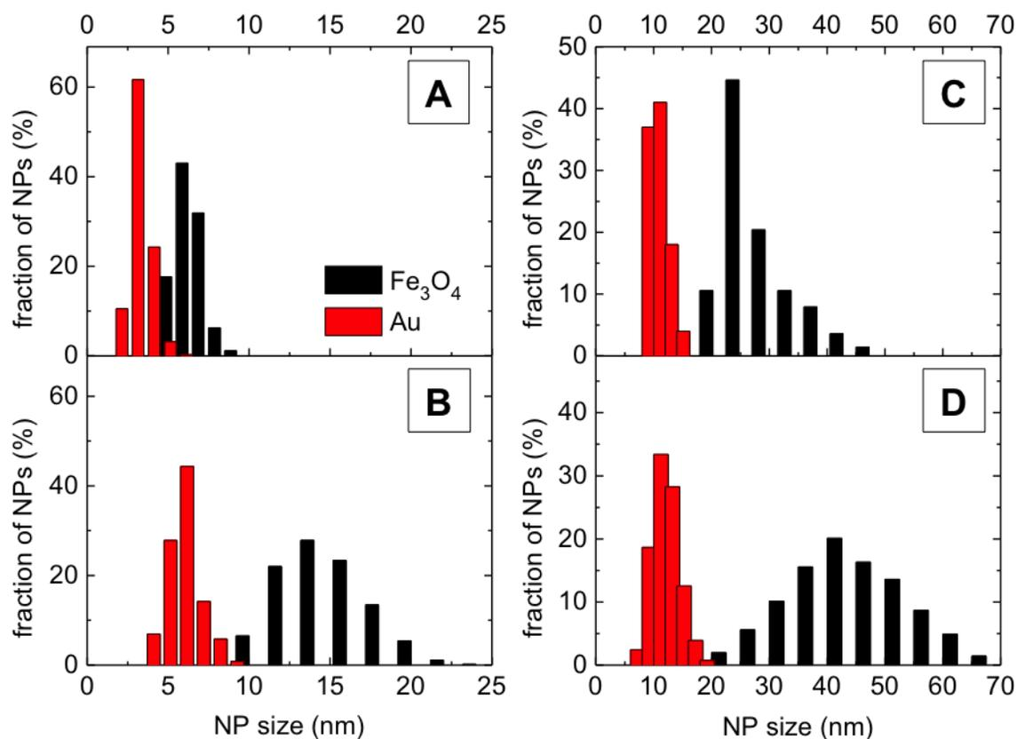
**Figure S1:** Size distributions calculated from TEM images of magnetite (black) and gold (red) parts of NPs for the samples with in situ synthesized Au seeds: A) MNP-6; B) MNP-15; and with pre-synthesized Au seeds: C) MNP-25; D) MNP-44.
