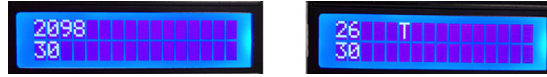
Fig. 8. VISTO display for an experiment where black and white displays alternate (left; experimental procedure in Fig. 6A), and when white displays are preceded by a trigger (right; experimental procedure in Fig. 6B). In both cases, the white display is presented for 30 ms. In the experimental paradigm shown on the left, the white display is preceded by a 2098 ms black display. In the experimental paradigm shown on the right, a trigger is presented 26 ms prior to the white display.
