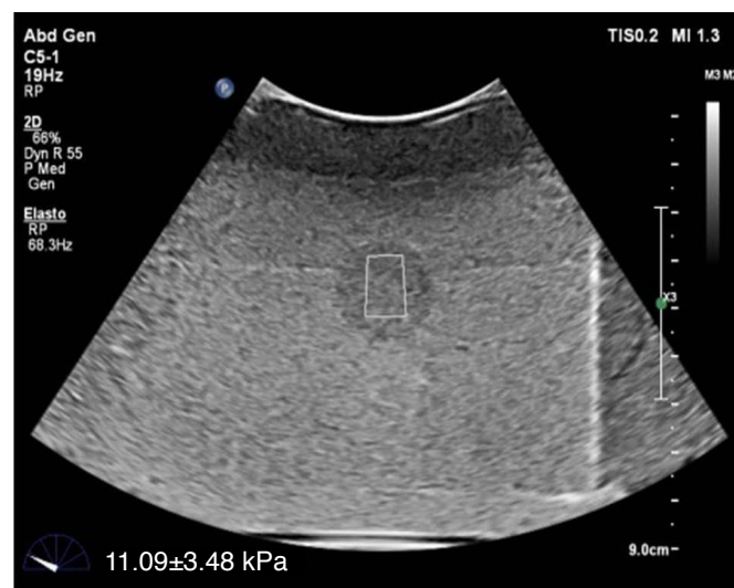
Fig. 2. Point shear-wave elastography (pSWE) of a lesion in an elasticity quality assurance phantom Model 049.
