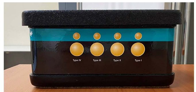
Fig. 1. Elasticity quality assurance phantom. Phantom Model-049 (Computerized Imaging Reference Systems, 2016). The phantom contains eight spherical inclusions with different stiffness values, diameter and depth.
