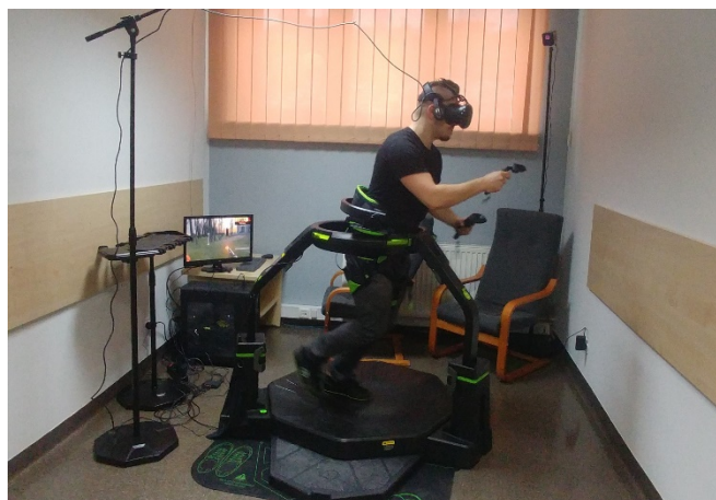
Figure 1. Omni-directional Omni treadmill enabling locomotive movements in virtual reality (VR). Source: author’s elaboration.
