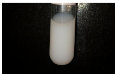
Figure 1. Essential oil nanoemulsion of P. heptaphyllum resin in hydrophilic-lipophilic balance 14 on day 0.
