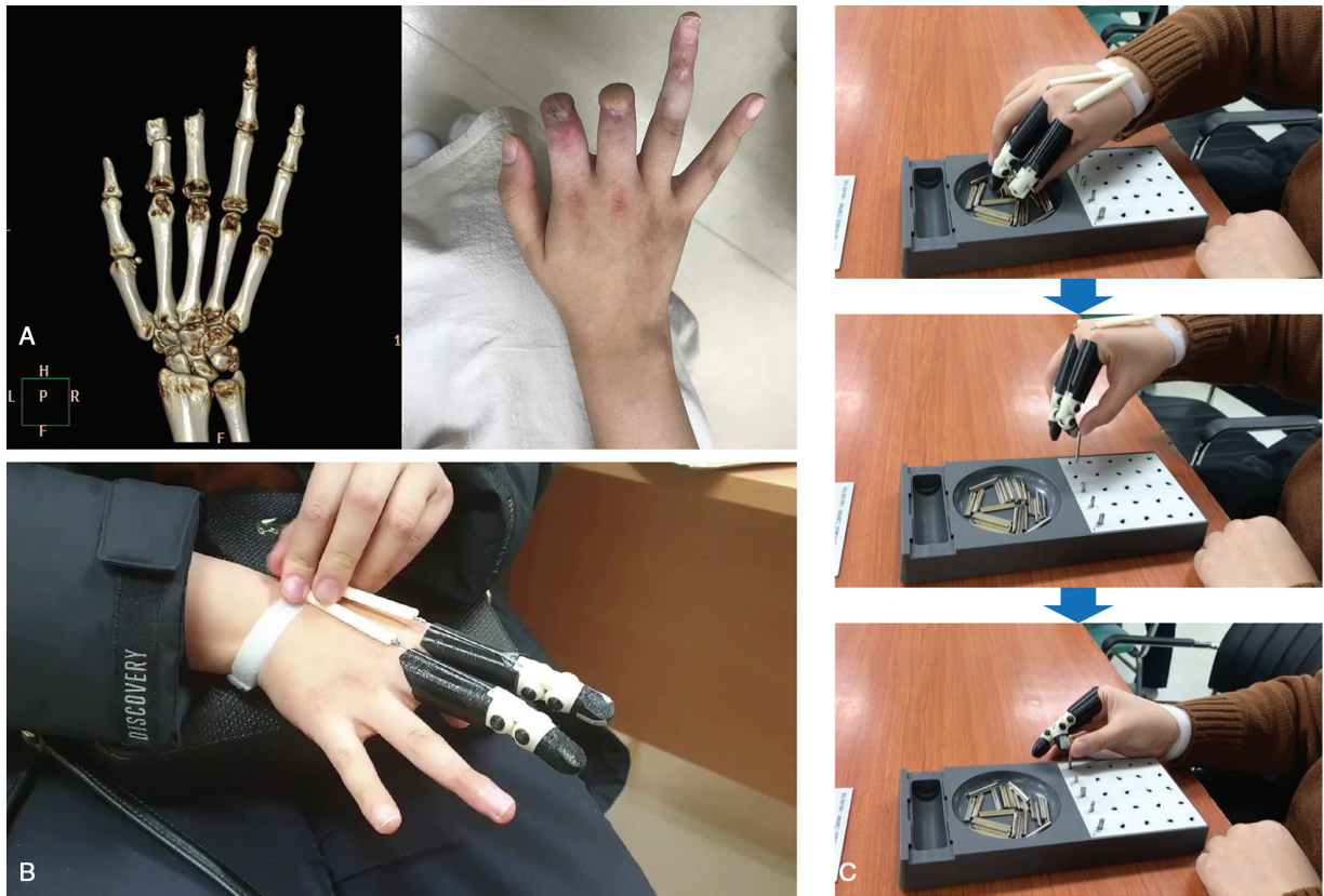
Figure 2. The case of patient 1. (A) A 3D-reconstructed bone structure from a computed tomographic scan and gross appearance of the right hand in patient 2. The amputation levels correspond to second and third proximal phalanges. (B) The patient is wearing the fabricated body-powered 3D-printed finger prostheses. (C) The patient is performing peg board training with the finger prostheses.
