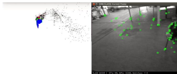
Fig 5. ORB-SLAM getting stuck in wrong initialization freiburg2_large_with_loop from TUM RGB-D dataset [19].
