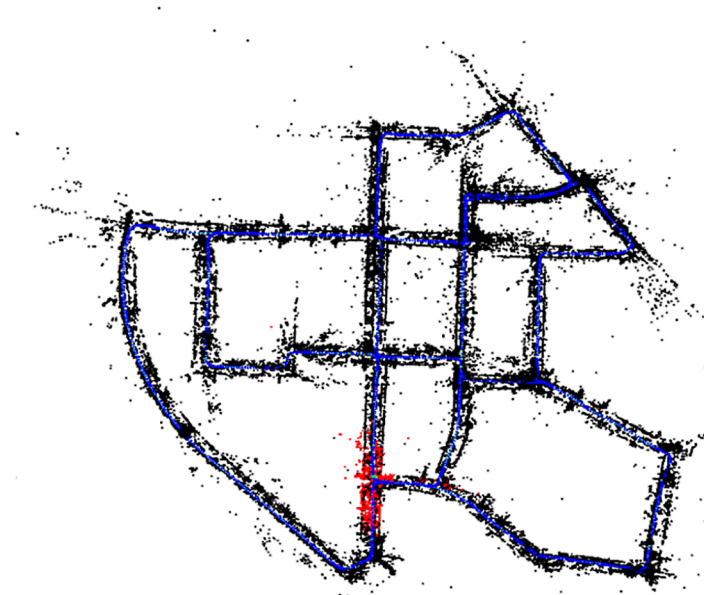
Fig 4. ORBSLAMM running on KITTI sequences 00 and 07 simultaneously. It took 494.2 seconds to get the final map which contains 1934 keyframes, with translation error of 1% of trajectory's dimensions.
