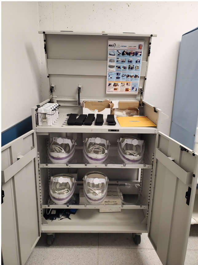
Fig. 2. CAPR® devices with charging stand allocated for dedicated use by the Otolaryngology Service.
