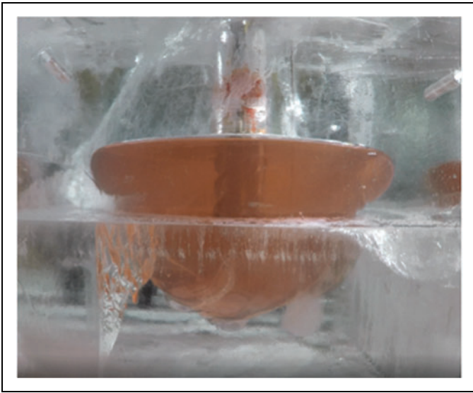
Fig. 4. RedWater undergoing testing in a block of water ice at -25^{\circ}\text{C} . Shown is a melt pool formed after \sim 2 h of melting while the auger bit ( center ) is being rotated to stir up the water. The pool is 10" in diameter and contains 15 L of water.
