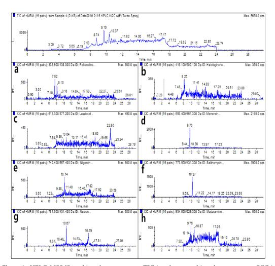
**Figure 2.** HPLC–MS/MS total ion chromatograms (TICs) and extracted ion chromatograms (XICs) (**a**–**h**: robenidine (ROB), halofuginone (HAF), lasalocid (LAS), monensin (MON), nigericin (NIG), salinomycin (SAL), narasin (NAR), and maduramicin (MAD)) of eight coccidiostats in a blank egg sample. Note: "Int ..." is represented as "Intensity, cps" in the figure, the following is the same.
