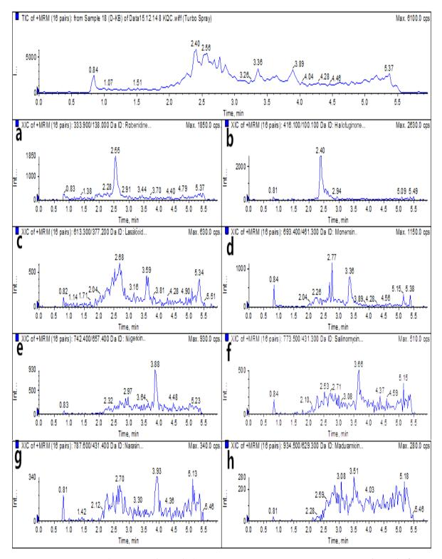
**Figure 3.** UPLC–MS/MS TICs and XICs (**a**–**h**: ROB, HAF, LAS, MON, NIG, SAL, NAR, and MAD) of eight coccidiostats in a blank egg sample.
