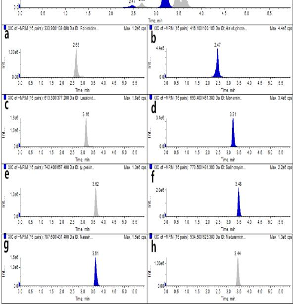
Figure 5. UPLC-MS/MS TICs and XICs (a-h: ROB, HAF, LAS, MON, NIG, SAL, NAR, and MAD) of a blank egg sample spiked with ROB and HAF at 25.0 µg/kg, MON at 37.5 µg/kg, MAD at 60.0 µg/kg, and LAS, NIG, SAL, and NAR at 15.0 µg/kg.
