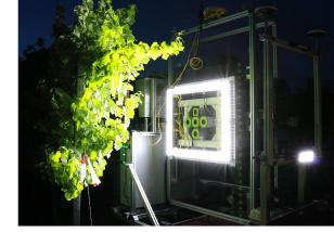
**Figure 4.** The PHENObot. RTK-GPS is attached at the top. A five camera system is attached on a camera movement frame to adjust the camera-canopy distance and camera height. The RGB camera in the middle of the camera system was used for our purposes. Around the camera system, the lighting unit is situated in a rectangular frame.
