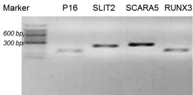
Figure 1. Electrophoresis results for pyrophosphate sequencing template. The target gene was amplified by using the primers based on the sulfite-treated pyrophosphate sequencing template. The results showed that p16 , Runx3 , SCARA5 , and SLIT2 pyrophosphate sequencing templates were successfully amplified. p16 =multiple tumor suppressor 1, Runx3 =human runt-related transcription factor 3, SCARA5 =scavenger receptor class A, member 5 putative, SLIT2 =secreted glycoprotein 2.
