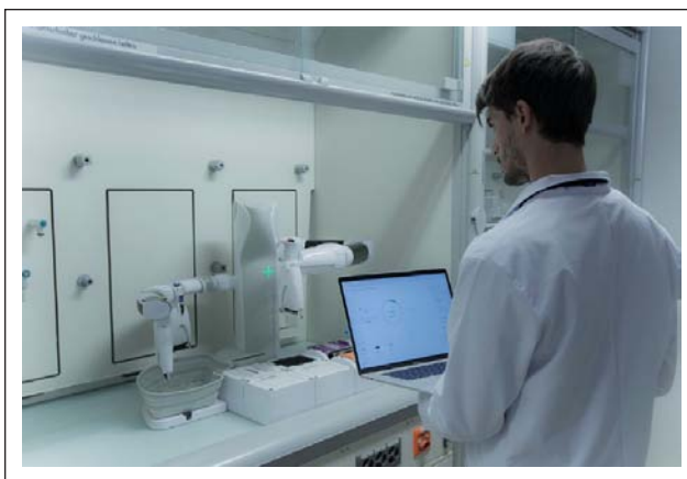
Figure 5. Andrew+ pipetting robot, in a laminar flow hood, being controlled by OneLab.
