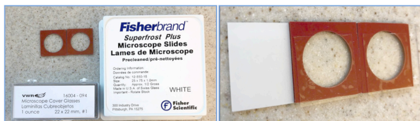
Figure 3. Construction of a Collagen Chamber
