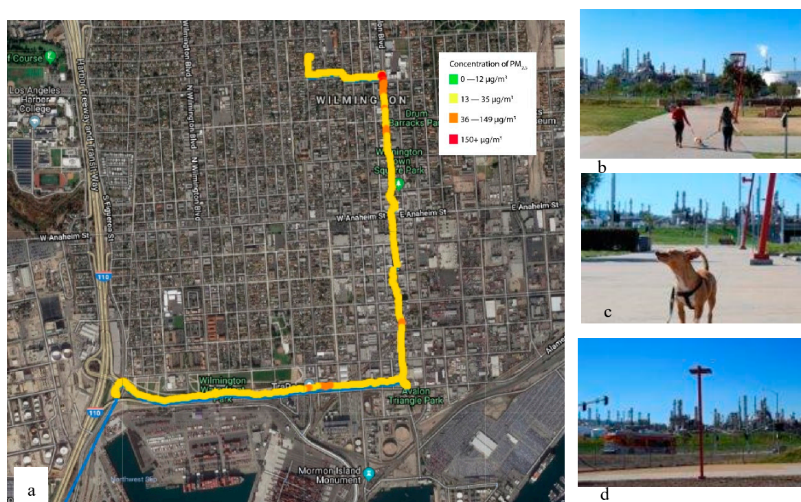
Figure 4. An example of the combination of images (all taken by the participant) with sensor data. (a) Map of youth air monitoring route recorded with AirBeam on AirCasting app. (b) A park adjacent to an oil refinery complex in Wilmington, CA. (c) The participants dog walking at the park. (d) A view of the industrial complex from the park. The participant describes the following: “I took part in a program with University of Southern California to help track the air quality in my community. After walking around Wilmington and San Pedro with an air monitor, I was surprised with the results. On the map shown, you are able to see one of my routes to school. The yellow and orange indicate the higher levels of fine particulate matter in the air. This was shocking to see. I decided to focus my images on the pollution happening around our parks. These are only two parks that are near my home, where the refineries are visible, and you can see the particulate matter in the air. Many babies, kids, adults, and even animals breathe in this pollution that causes serious damage to one’s health. That is why I am in CBE [Communities for a Better Environment], to make a difference in my community and to stop this from getting any worse.”
