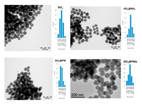
Figure 2. TEM images and diameters distribution of SiO<sub>2</sub>, SiO<sub>2</sub>@PH<sub>2</sub>, SiO<sub>2</sub>@PW and SiO<sub>2</sub>@PMo beads.
