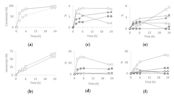
**Figure 8.** (a) Comparison of Lim conversion between (a)  $H_3PW_{12}O_{40}$  (□) and  $SiO_2@PW$  (○), (b)  $H_3PMo_{12}O_{40}$  (□) and  $SiO_2@PMo$  (○). Evolution of *trans*-LO (△), *cis*-LO CHD (♠), eq-LD (♠), ax-LD (○),  $C^{ol}$  (⋄) and  $C^{one}$  (♠) with (c)  $H_3PW_{12}O_{40}$ , (d)  $H_3PMo_{12}O_{40}$ , (e)  $SiO_2@PW$  (Run 1) and (f)  $SiO_2@PMo$  (Run 1).
