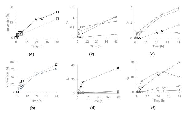
**Figure 7.** Comparison of conversion of CH between (a)  $H_3PW_{12}O_{40}$  (□) and  $SiO_2@PW$  (○), (b)  $H_3PMo_{12}O_{40}$  (□) and  $SiO_2@PMo$  (○). Evolution of CHO (△), CHD (×), CHol (□) and CHone (●) with (c)  $H_3PW_{12}O_{40}$ , (d)  $H_3PMo_{12}O_{40}$ , (e)  $SiO_2@PW$  (Run 1) and (f)  $SiO_2@PMo$  (Run 1).
