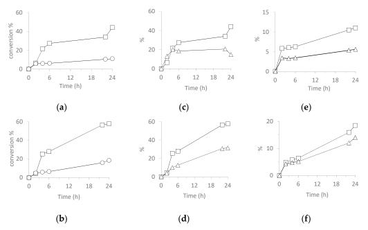
**Figure 9.** Comparison of  $CY^{ol}$  conversion between (a)  $H_3PW_{12}O_{40}$  ( $\square$ ) and  $SiO_2@PW$  ( $\bigcirc$ ), (b)  $H_3PMo_{12}O_{40}$  ( $\square$ ) and  $SiO_2@PMo$  ( $\bigcirc$ ). Conversion of  $CY^{ol}$  ( $\square$ ) and formation of CYone ( $\triangle$ ) with (c)  $H_3PW_{12}O_{40}$ , (d)  $H_3PMo_{12}O_{40}$ , (e)  $SiO_2@PW$  (Run 1) and (f)  $SiO_2@PMo$  (Run 1).
