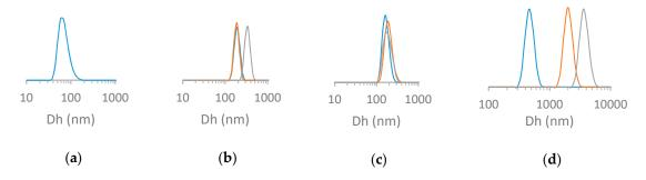
**Figure 1.** Size (hydrodynamic radius) distribution (in number) obtained by DLS for the  $SiO_2$  (a)  $SiO_2@NH_2$  (b)  $SiO_2@PW$  (c) and  $SiO_2@PMo$  (d) beads. The time dependent size increase (case b–d) has been indicated by the different colors (blue-orange-grey).
