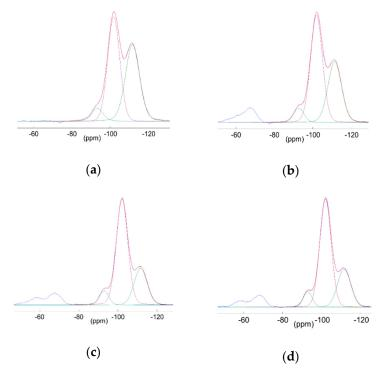
Figure 5.  $^{29}$ Si CP MAS NMR spectra of SiO<sub>2</sub> (a), SiO<sub>2</sub>@NH<sub>2</sub> (b), SiO<sub>2</sub>@PW (c) and SiO<sub>2</sub>@PMo (d).
