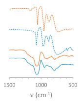
**Figure 4.** From up to down: Relevant IR vibration area for  $H_3Pmo_{12}O_{40}$ ,  $H_3PW_{12}O_{40}$  and difference spectra (SiO<sub>2</sub>@Pmo-SiO<sub>2</sub>@NH<sub>2</sub>) and (SiO<sub>2</sub>@PW-SiO<sub>2</sub>@NH<sub>2</sub>).
