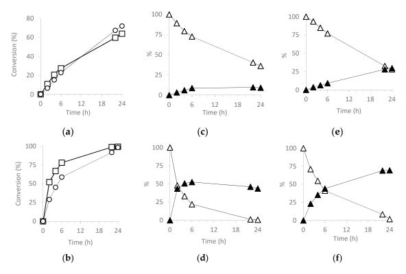
Figure 6. Comparison of CO conversion between (a)  $H_3PW_{12}O_{40}$  ( $\square$ ) and  $SiO_2@PW$  ( $\bigcirc$ ), (b)  $H_3PMo_{12}O_{40}$  ( $\square$ ) and  $SiO_2@PMo$  ( $\bigcirc$ ). Evolution of CO ( $\triangle$ ) and COE ( $\blacktriangle$ ) with (c)  $H_3PW_{12}O_{40}$ , (d)  $H_3PMo_{12}O_{40}$ , (e)  $SiO_2@PW$  (Run 1) and (f)  $SiO_2@PMo$  (Run 1).
