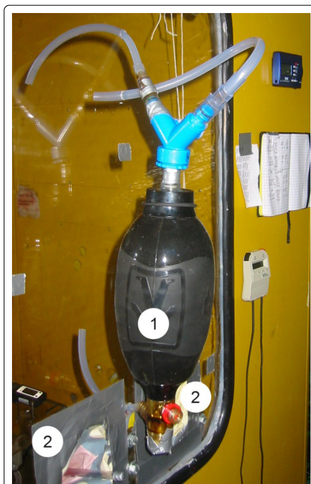
Figure 1 Picture taken from outside of the testing chamber (telephone cabin) showing the ETSE (1) and the glove ports (2).
