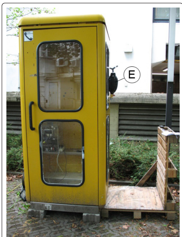
Figure 2 Testing chamber (telephone cabin) with outside mounted ETSE (E).
